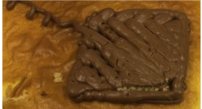
Figure 5. Pressure release test for a 50 mm 2 square shape.
