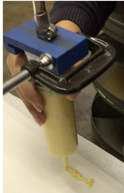
Figure 2. Preliminary conceptual design for extrusion testing.
